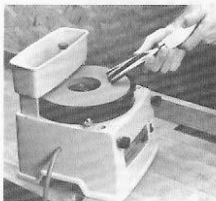
Figure 3. Using the 9820-2 sharpener for freehand sharpening of a carving gouge.
