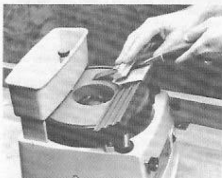
Figure 2. Highland Jig used with 9820-2 for accurate sharpening of a chisel.
