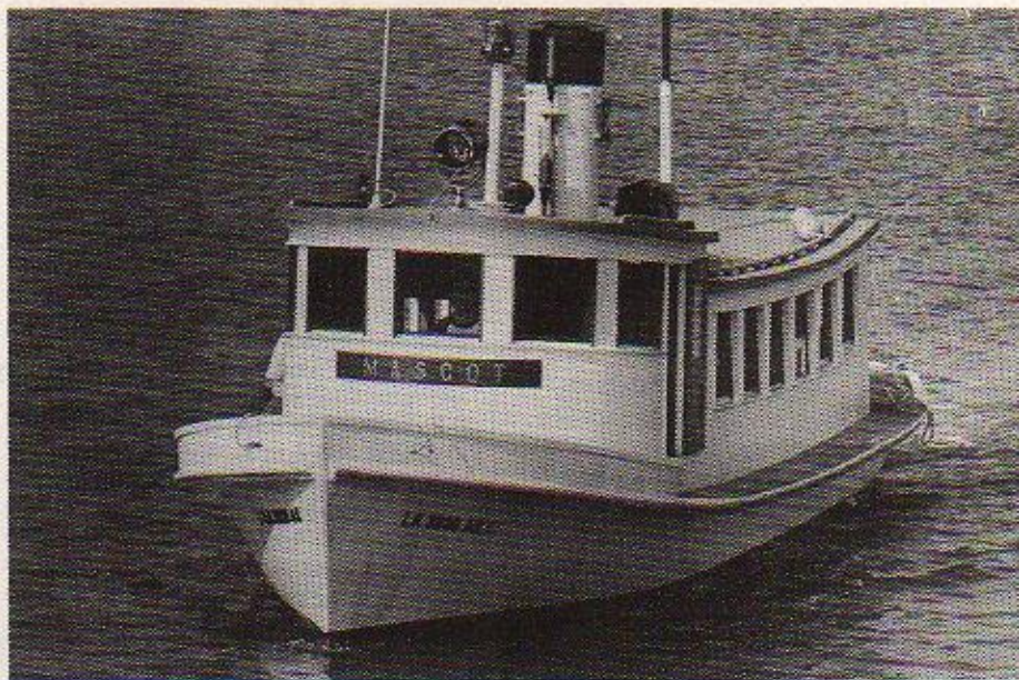
Dufrene built William Ellsworth's 30-foot steam launch "Mascot" in 1969. He later cut it in two and extended it to 39 feet. Photo by Bevil S. Knapp
