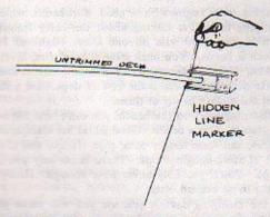
where the cumber which I'll call a Hidden Line Marker is used where the cumber to be followed cannot be seen, but is interrupted by the piece you are marking such as trimming a deck to follow the sheer curve. These gadgets are easy to make and I usually have one or two laying around ready to use. Just glue two tongue depressors, or sucker sticks, to a scrap of pine about an inch thick. Since these fingers are of equal length, one will always be over the other and will mark the same
