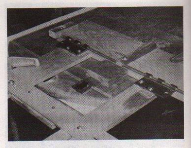
In photos above and below, jig is in position to flush mount a table-leaf hinge.
