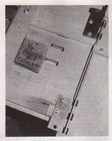
Adjust the jig with the spacer block for the two remaining cutting lines. To remove the mortised workpiece and insert a new workpiece, remove only the one clamp at the cavity opening. If the mortises on a frame are off center, the stop board assembly should be reversed on the jig in order to cut the second mortise on each frame workpiece.
