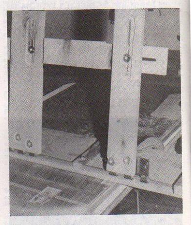
Each hinge is screwed into T-nuts in the bottom of two narrower straight edges (2-1/2" x 13") which then slide perpendicular to the base straight edge. To insure that the straight edges of these boards and the base are on the same plane, insert shims as necessary under each leaf. Use screws with a diameter smaller than the hinge leaf screw holes. This will enable you to finely adjust the three straight edges to form two 90° angles.
