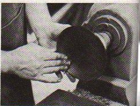
Wet sanding the inside of the paten. No heavy sanding was necessary.
