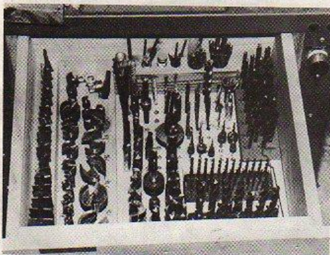
Drawers are compartmentalized and fitted for specific types of tools. Above, long narrow slots accommodate carving tools and chisels. Below, the base of the drawer has been bored to hold every kind of drill bit. At bottom, a deep drawer provides easy selection of sawblades and grinding stones.
