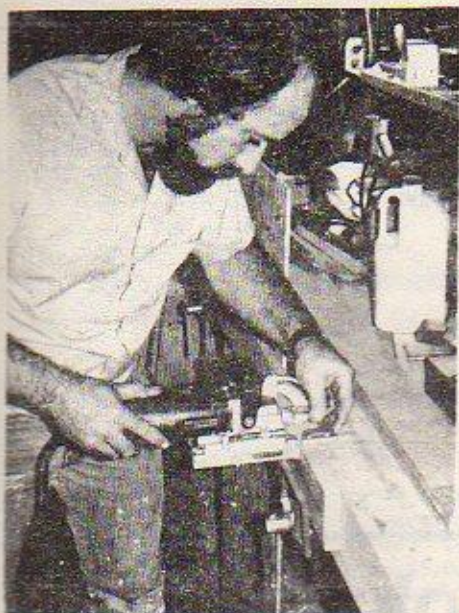
First the Lamello was used to cut matching grooves along the four sides of all pieces to be connected. A pencil-marked template was held in the vise next to the piece to be grooved.
